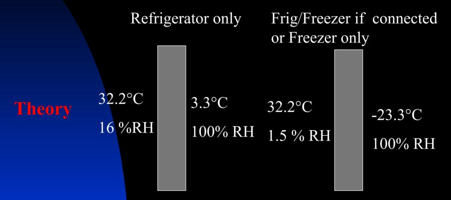
Half barrier film area at hot wall condition and half at the cold wall condition
